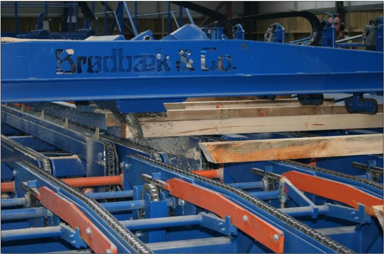
The weather top saw unit in action
